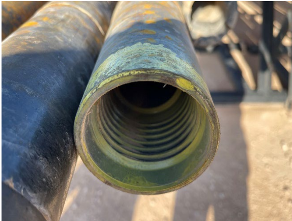
Reject Box Stabbing Damage
