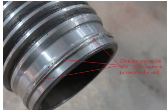
Pin Bump Seal Galling - Not Repairable
