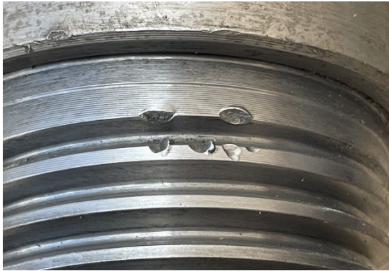
Bring connection into compliance by remove raised edges
