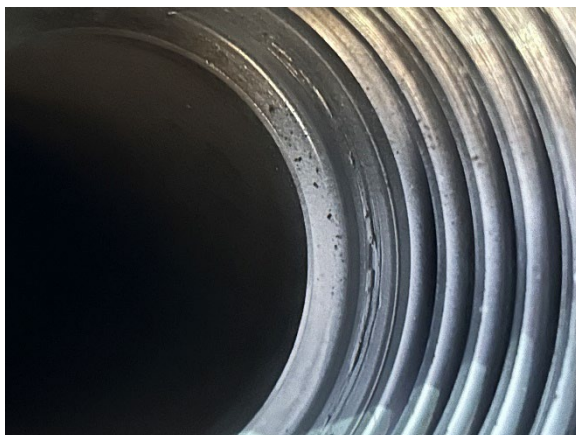
Box seal galled, torque shoulder okay
