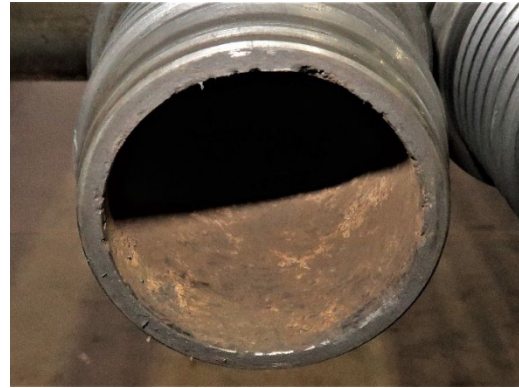
Likely Acceptable Sharp Corners Must be Removed
