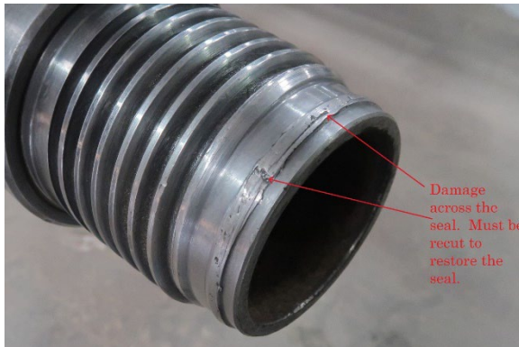
Pin Bump Seal Galling - Not Repairable
